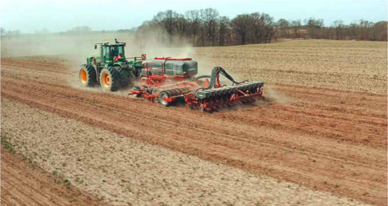
The HORSCH Maestro RV can be linked directly to the tractor or to a seed wagon. In the video, Arkadiusz Grzech explains why he chose the combination with the Focus TD.
