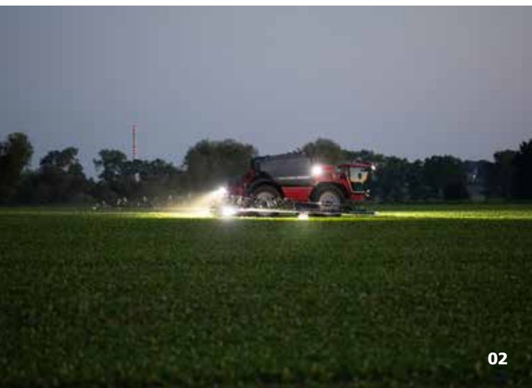
01 Thistle nest in sunflowers (5x5 m) 02 Final treatment in sugar beet with a HORSCH Leeb PT using the SpotSpraying method
